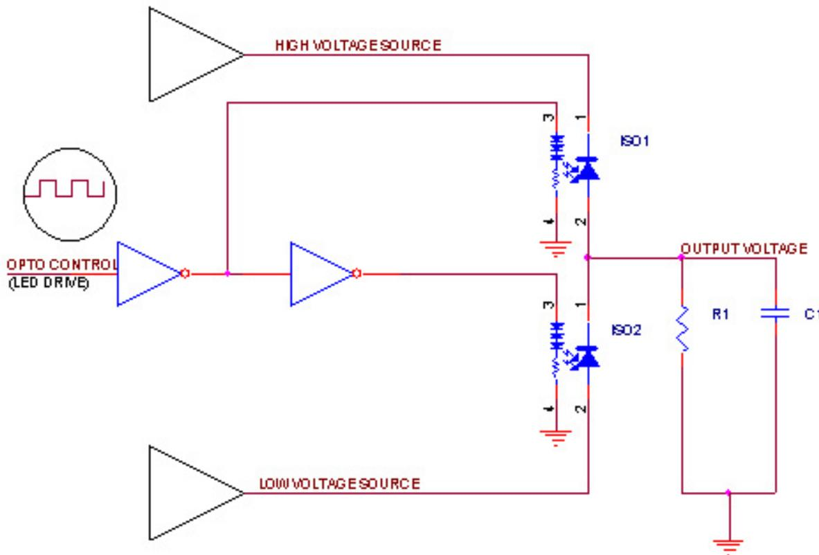
Figure 3: Switching using OC250 optocoupler solid state relays
