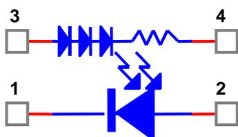
*Figure 2: Representation of OC250 optocoupler solid state relay.*
